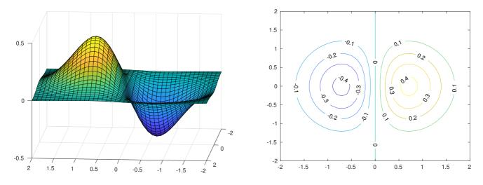
(a) Surface plot of an SVM classifier composed by two Gaussians with (b) Contour plot of an SVM classifier composed by two Gaussians with weight -1 and 1. Equivalent to a binary linear classifier.
