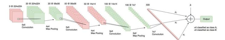
Fig. 4: Architecture of the original CNN model in binary classification
