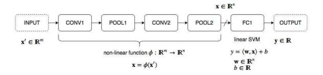
Fig. 1: An example CNN which can be viewed as a non-linear function  $\Phi$  and a linear SVM classifier. During training, the output is fed to a loss layer where it is compared with ground truth.
