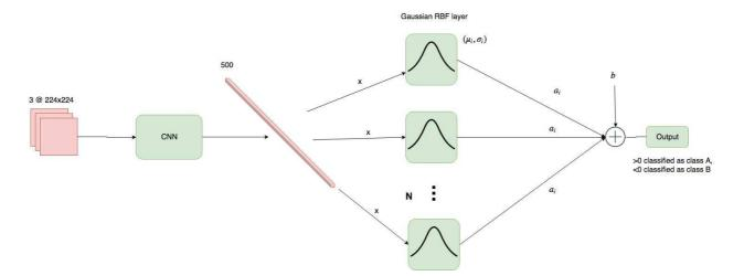
Fig. 5: Architecture of the proposed model combining CNN and RBF-kernel SVM. In our experiments, N = 2 or N = 20.
