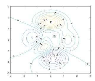
(b) Contour plot of an SVM classifier composed by five Gaussians. Level 0 indicates the separating plane. One can see that this classifier is able to separate data that is not linearly-separable.
